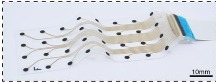
soft ECoG SP Lacour – EPFL / Neurosoft Bioelectronics
